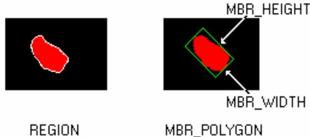
**Fig. 4.8.** Object parameterization by means of the minimum bounding rectangle (MBR).
