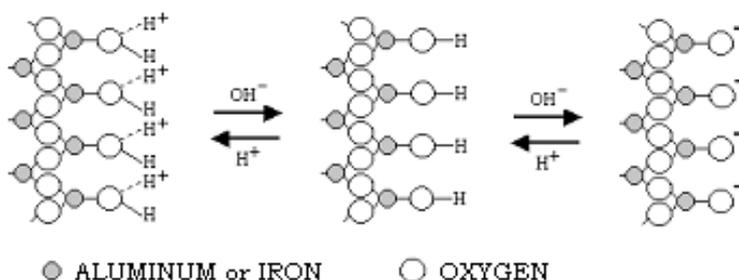
*Fig. 77. Formation of variable charge on surface of aluminum and iron oxides.*
