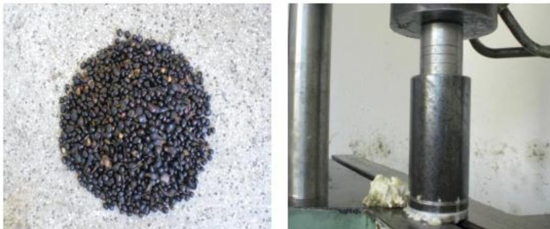
Fig. 1. Compression test of heat-treated palm kernels showing caked kernel oil (Kabutey et al., 2012)
